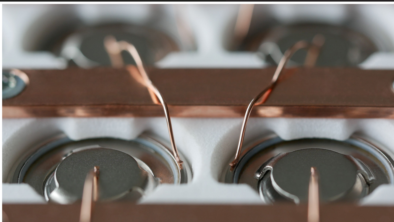
Figure 1 Contacting Battery Cells with Copper Wire Bonding
