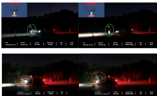
Images show vehicle with lidar-based emergency braking stopping before adult target @ 50% overlap (above) and vehicle with camera and radar-based solution only crashing into adult target (below)
