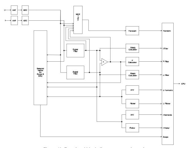
Figure 49: Functional block diagram computing unit
