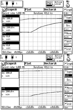
Figure 28: Scope display with split off/on
