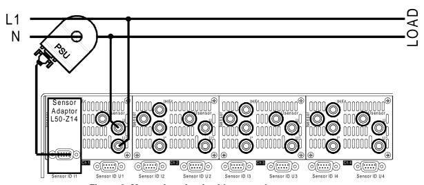
Figure 8: Measuring circuit with external current sensor
