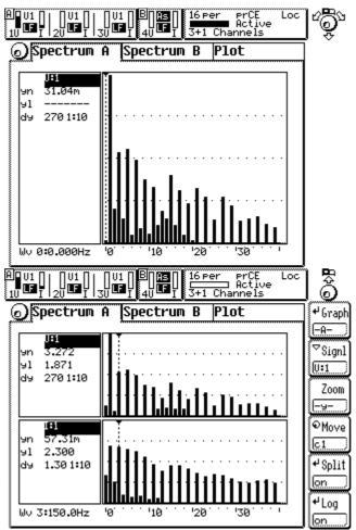
Figure 35: Graphical display of harmonics
