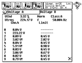
Figure 33: Display of voltages in CE-Harm-Harm mode
