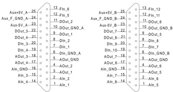
Figure 44: Processing Signal Interface Connector A and B
