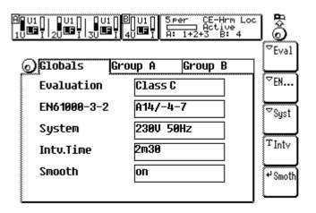
Figure 32: Measuring menu in CE-Harm mode
