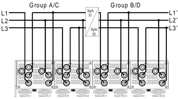
Figure 7: Measuring circuit for measuring efficiency (3/3phase)
