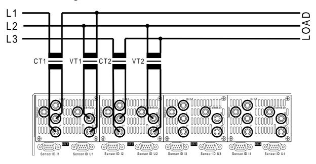
Figure 6: Measuring circuit with current and voltage transformers in Aron wiring
