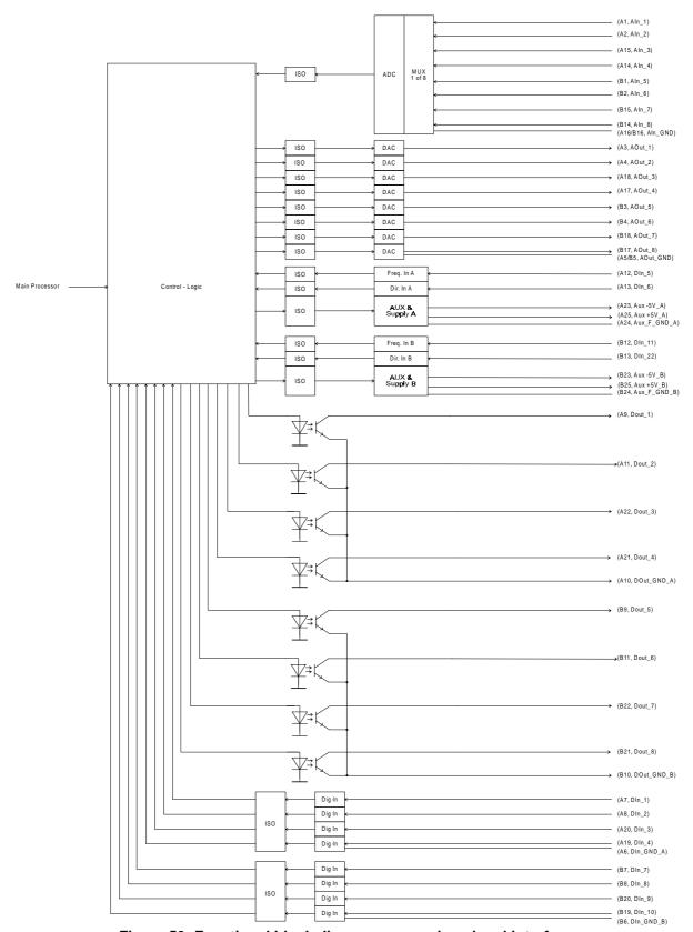
Figure 50: Functional block diagram processing signal interface
