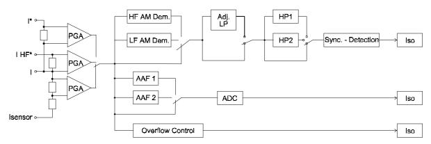
Figure 48: Functional block diagram current channels
