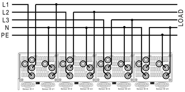
Figure 3: Measuring circuit 3 phase system with neutral
