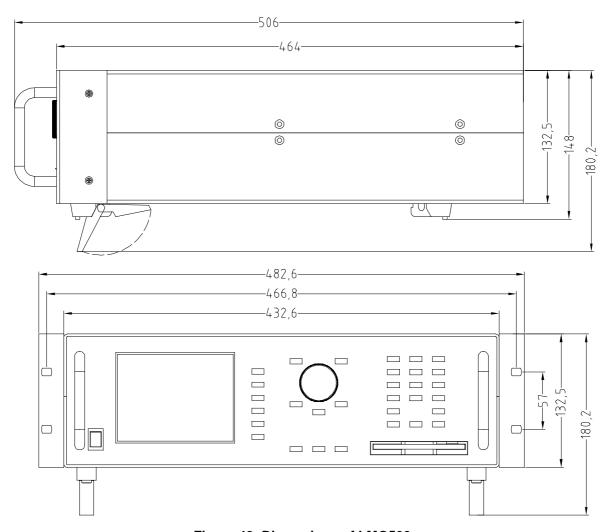
Figure 42: Dimensions of LMG500
