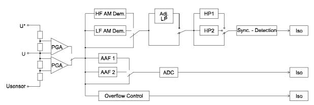
Figure 47: Functional block diagram voltage channels
