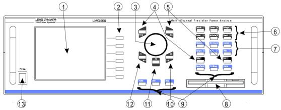
Figure 12: Front panel of the instrument
