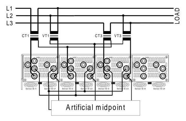
Figure 10: Measuring circuit for measuring in middle and high voltage sytems without N
