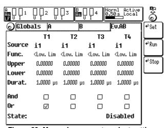
Figure 23: Measuring menu, transient settings
