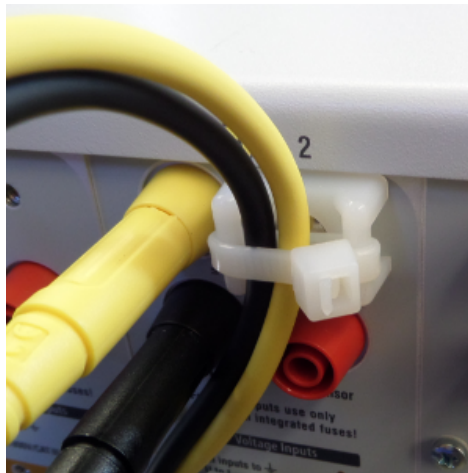
Figure 5.24: screw mounted cable tie mounts
