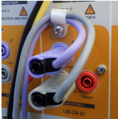
Figure 5.23: screw mounted cable clamps
