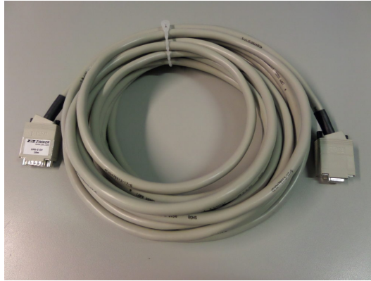
Figure 5.9: Shielded DSUB9 extension cable
