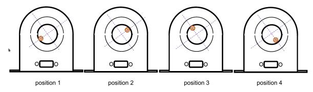
Figure 4: Influence from the conductor centering
