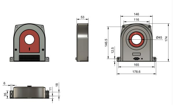
Figure 2: PCT1200 mechanical dimensions, all dimensions in mm, positive current direction is identified by an arrow on the transducer body
