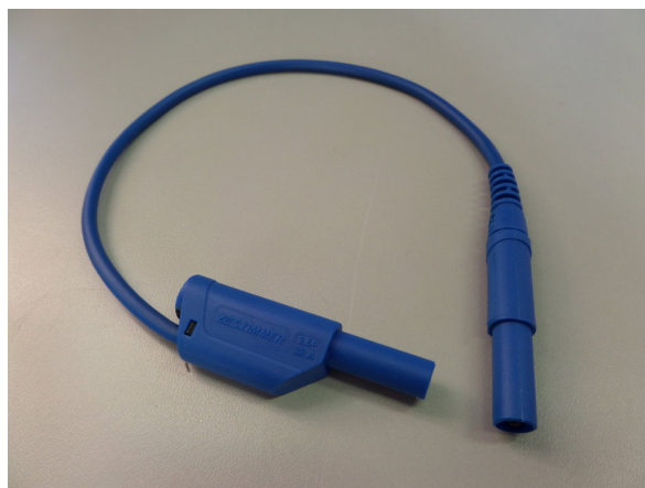
Figure 5.19: Safety laboratory lead for general purpose
