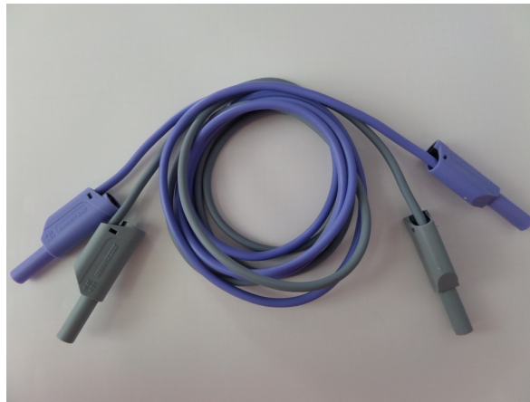
Figure 5.17: Safety laboratory leads for current path
