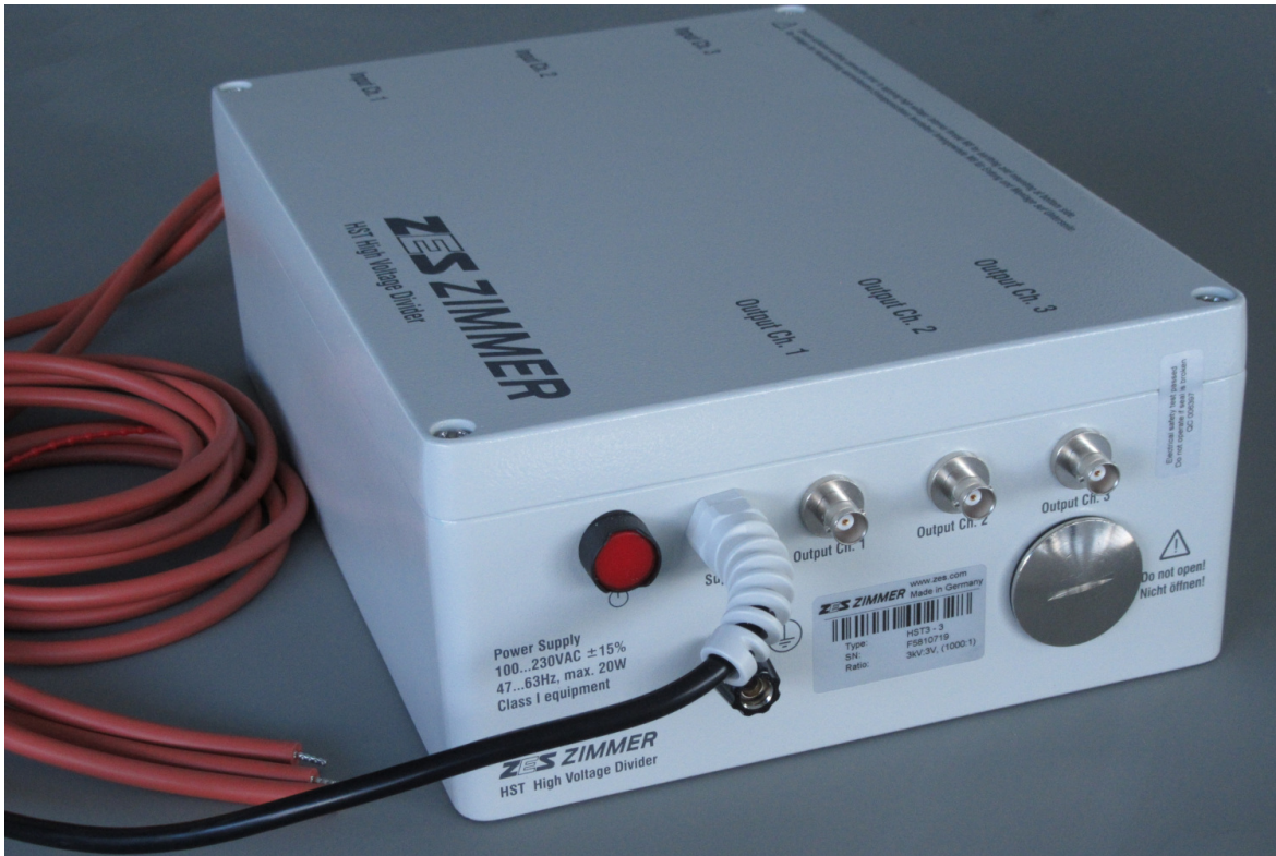
Figure 3.1: Precision high voltage divider
