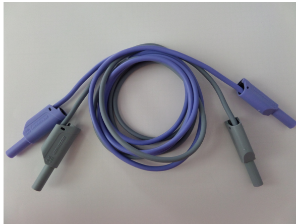
Figure 5.15: Safety laboratory leads for current path
