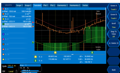
Simultaneous measurement of narrow and broadband values
