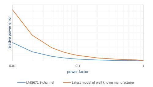
Figure 3: Power accuracy vs. power factor / 230Vrms, 2.5Arms, 50Hz
