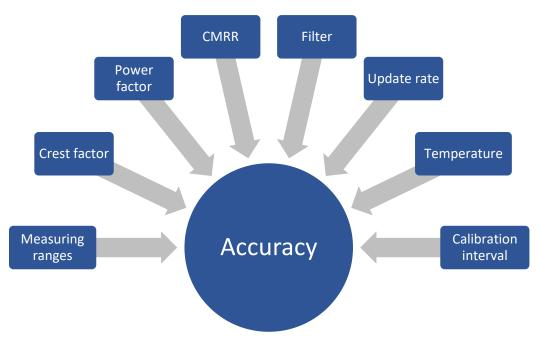
*Figure 1: Factors that influence the measuring instrument's accuracy*
