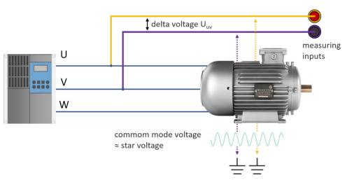
Figure 4: Common mode voltage at the inverter output
