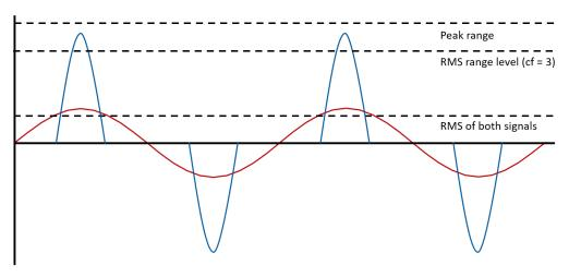
Figure 2: Comparison of two signals with same RMS value and different crest factors
