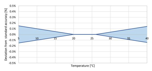
Figure 5: Deviation from standard accuracy vs environmental temperature for the LMG600 series
