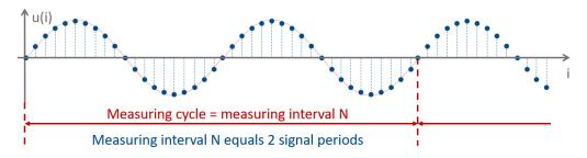
Figure 6: Cycle time respectively the measuring interval
