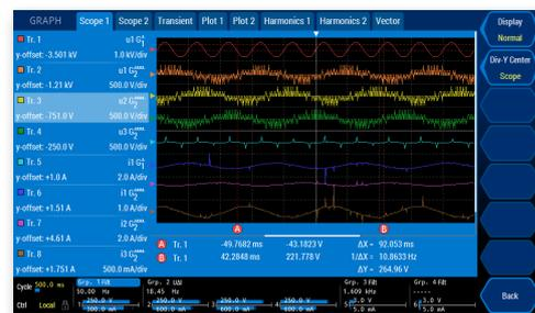
*Display of sampling values for 8 signals in two scopes*
