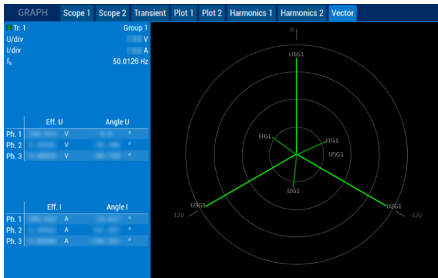
Figure 13: Vector diagram - extract from LMG671 Scope menu for checking phase symmetry
