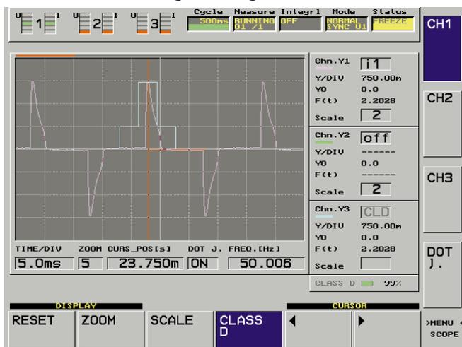
The menu in the figure beneath shows an emission of harmonics in relation to its limits. Current I1 is examined according the limits of instrumentation class D. The harmonics of the current are shown as red bars, the related limits as green bars. For better visualisation the
