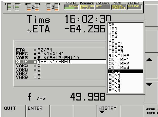
Using the integrated **formula editor** the user can build new values (VARiables) from all measured and computed values. The signals from the processing signal interface can be computed in the formula editor in the same way. All fundamental arithmetics are available, also more complex operations such as  $\sqrt{\quad}$ , sin and arcsin.
