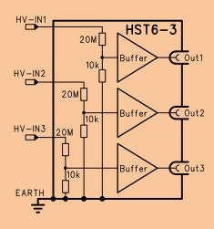
3-channel HST for three-phase systems (inverters)
