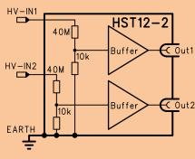
2-channel HST for floating voltages (difference measuring)
