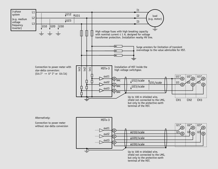
On the high voltage side the HST inputs in1, in2, in3 are connected with lines L1, L2, L3. All voltage measurements have the same reference potential: earth.
