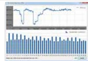
The tests performed by LMG Test Suite are in accordance with the currently valid edition of EN 61000-3-2/-12 or EN 61000-3/-11, and measurements according to ECE R-10.4 Annex 11 (electromagnetic compatibility of vehicles), for example, are also possible.
