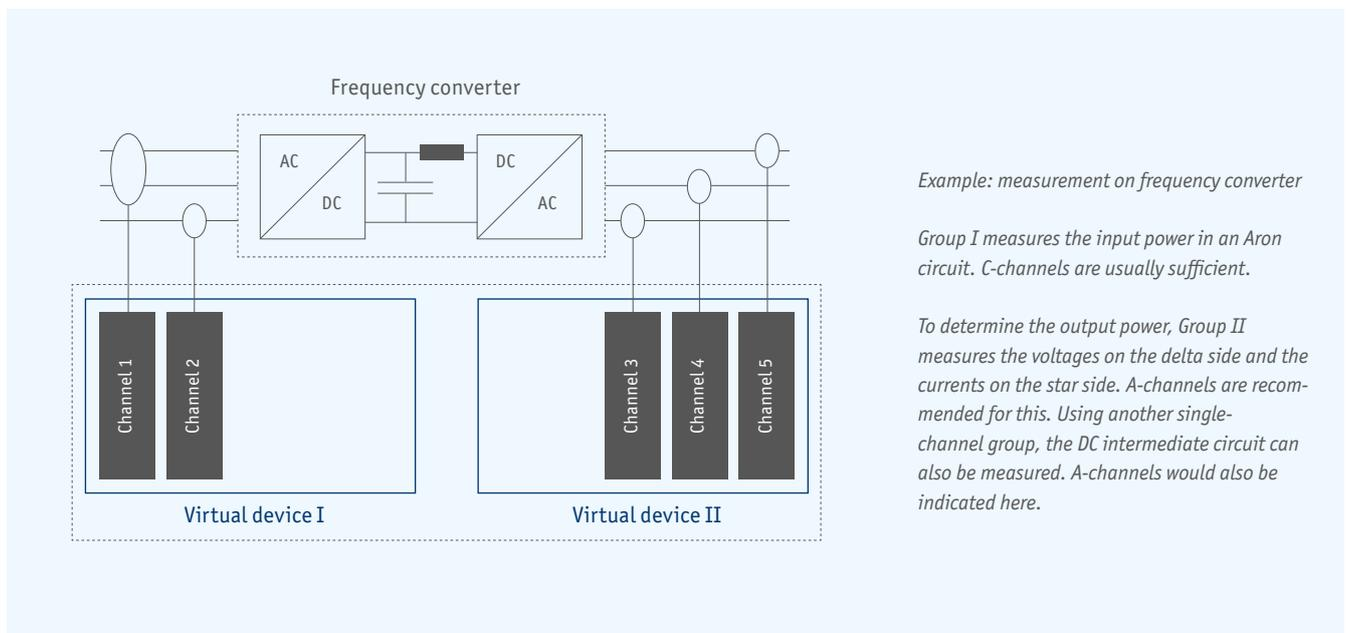
Example: measurement on frequency converter
