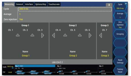
This screenshot depicts an example for logical grouping of an LMG600 fitted with 7 power channels, e.g. for measuring an electric drive. Group 1 & 2, with three channels each, could comprise the 3-phase input/output connections, while the single-channel Group 3 might represent the DC link.
