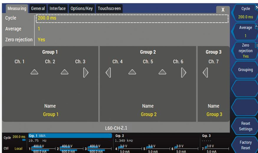
This screenshot depicts an example for logical grouping of an LMG600 fitted with 7 power channels, e.g. for measuring an electric drive. Group 1 & 2, with three channels each, could comprise the 3-phase input/output connections, while the single-channel Group 3 might represent the DC link.
