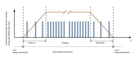
Energy meter pulses captured and energy measured by the LMG600 power analyzer
