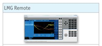
The LMG Remote PC software allows to easily control the LMG600 remotely from a Windows PC. Since this software mimicks the measuring device itself down to the last detail, the LMG600 can be operated as usual, even from the PC - no rethinking required, no familiarization time.
