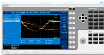
The LMG Remote PC software allows to easily control the LMG600 remotely from a Windows PC. Since this software mimicks the measuring device itself down to the last detail, the LMG600 can be operated as usual, even from the PC - no rethinking required, no familiarization time.
