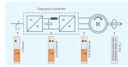
Determining the efficiency of an electric drive system
