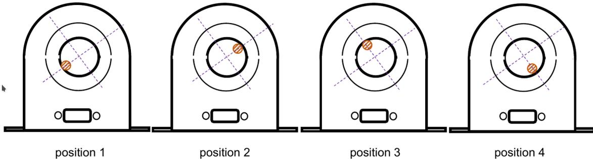
Figure 4: Influence from the conductor centering
