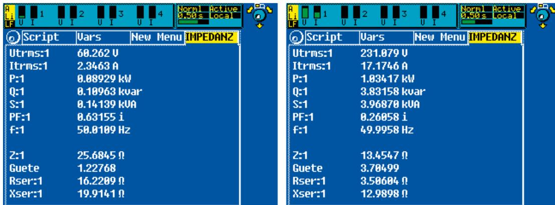
Picture 4: User-defined impedance menu of the LMG500 power analyzer
