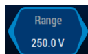
Figure 7.7: A disabled soft key which still displays a state. Although similar to the soft key in Figure 7.6 [→147], this soft key displays the current setting. This happens usually in conjunction with automatic functions. In this example, the auto-ranging mechanism is active, so it is not possible to manually change the range but the soft key provides information on which range was selected.
