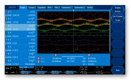
Display of sampling values of 8 signals in two scopes
