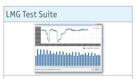
The tests performed by LMG Test Suite are in accordance with the currently valid edition of EN 61000-3-2/-12 or EN 61000-3/-11, and measurements according to ECE R-10.4 Annex 11 (electromagnetic compatibility of vehicles), for example, are also possible.
