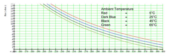
For temperatures above 65 degrees Celsius it is important not to exceed 200 Arms and 300A peak or 200A DC and a maximum measurement resistor value of 3 Ohm.
