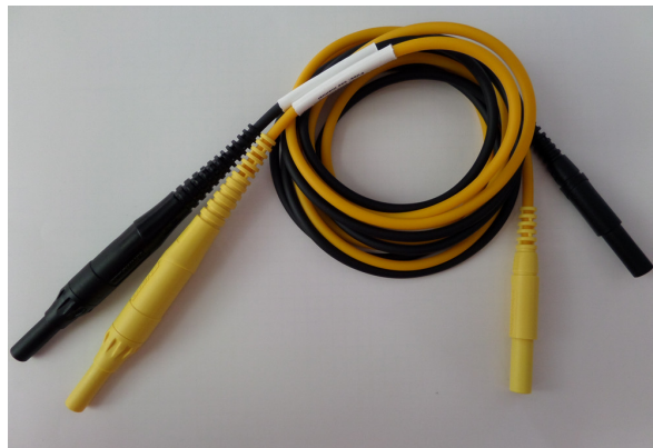
Figure 5.18: Fused safety laboratory leads for voltage path
